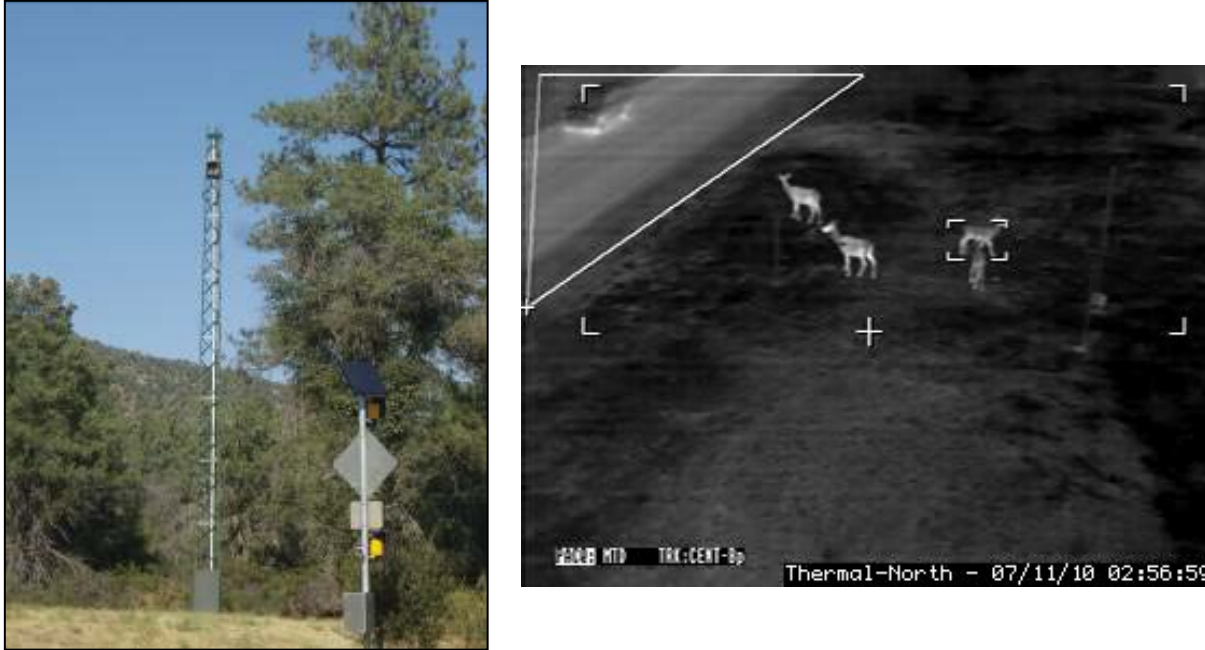
Figure 4.4. Tower-mounted infrared detection camera (left) and images of elk captured on target acquisition software (right).
