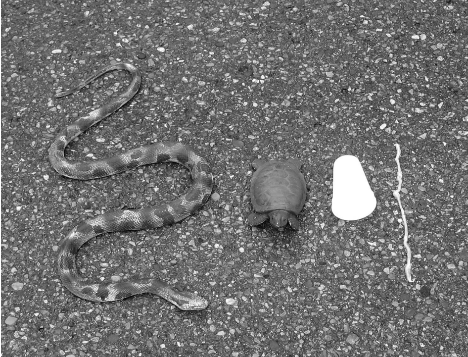
Figure 1. Picture of decoy snake, decoy turtle, Styrofoam cup, and grease control line that were individually placed on the center line of the road to determine incidence of intentional vehicle strikes.
